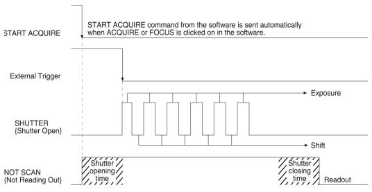
Figure 44. Single Trigger Timing Diagram
